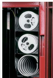
Spiral compartment for exchange spirals in case of product change
